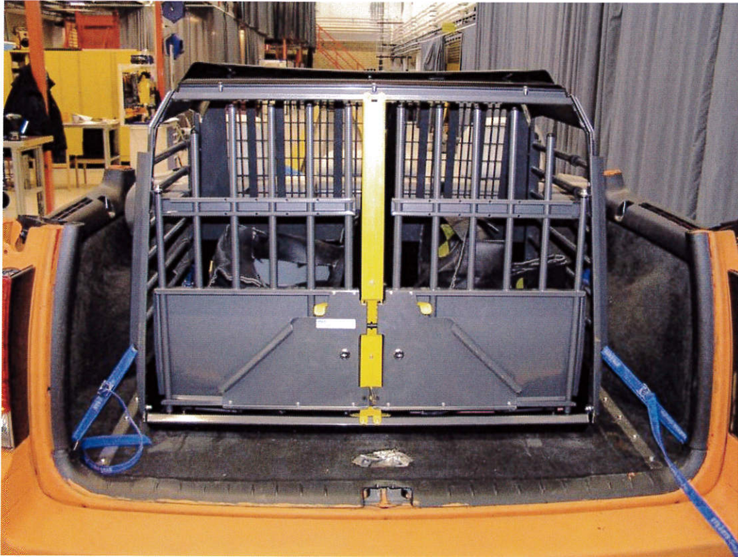
05 – After test, rear impact
