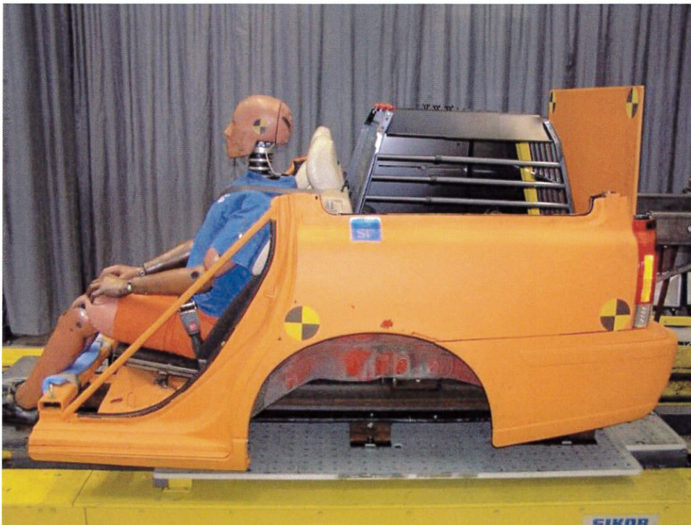
Figure 2 Test setup Rear impact test
