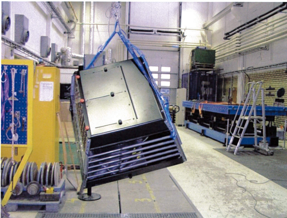
Figure 3 Test setup Drop test
