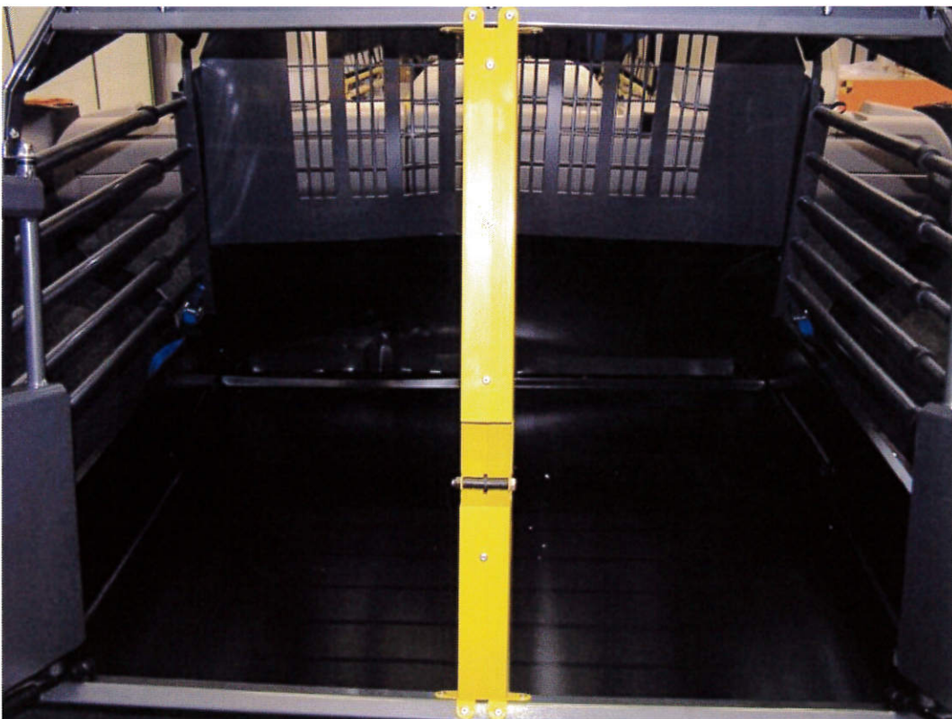
06 – After test, frontal impact
