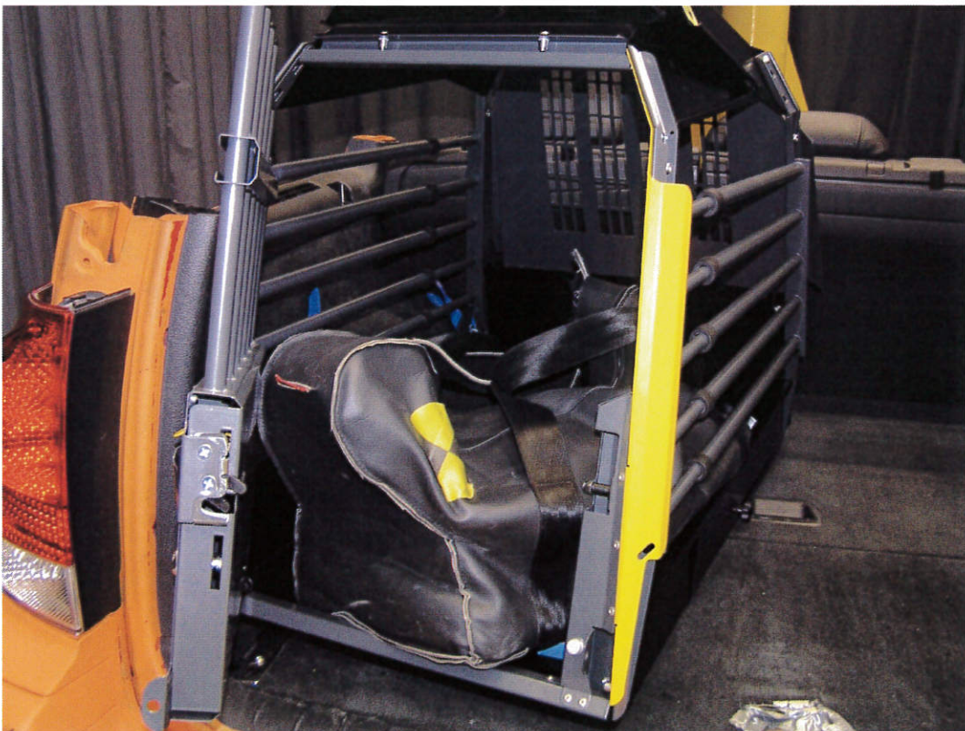
06 – After test, frontal impact
