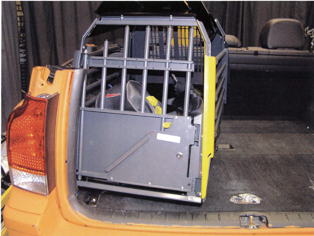
05 – After test, frontal impact
