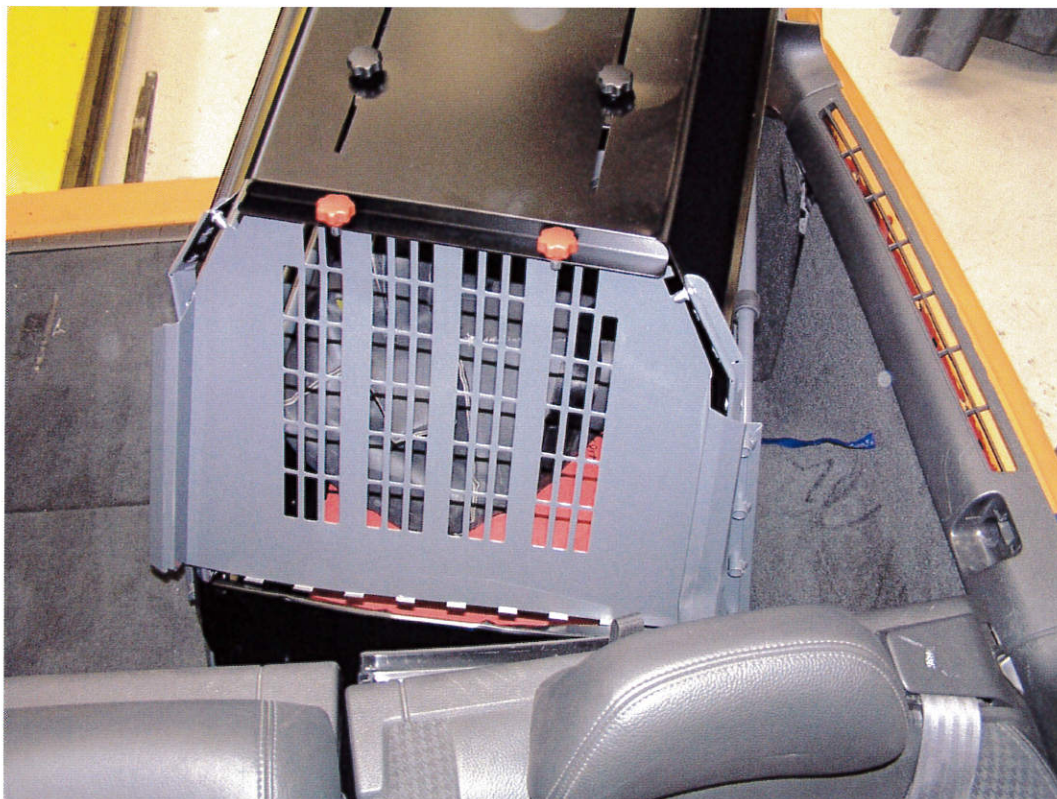
07 – After test, frontal impact
